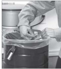
**Step 3:** Place the portion of the plastic bag around the Air Channel under the bag clip.
