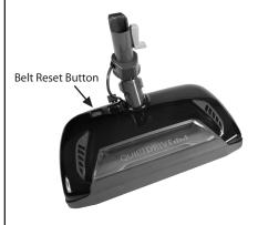
To correct problem: Turn off and unplug the powerhead, remove obstruction, then press belt reset button. If the problem persists, have the powerhead serviced by a Sears or other qualified service agent.
